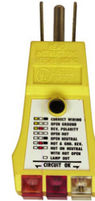
Typical 3-prong tester with GFCI trip button
